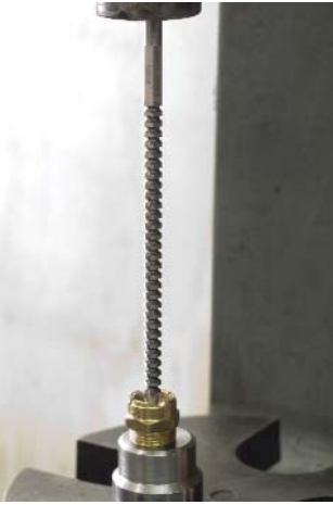
An automatic broaching operation using Hassay Savage one pass broaches.
